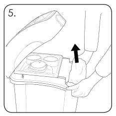
Release each sack individually from the bin rim and lift upwards out of the Bin Body. Return the Cradle to the centre.
